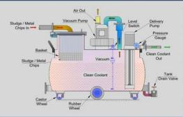
Oilmax Coolant / Sump Cleaner removes sludge, metal chips & swarf from Coolant tanks & filters it via reusable stainless steel mesh filter.
